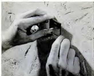
Mirror cemented to wall will help you decide whether dampness is condensation or seepage.
